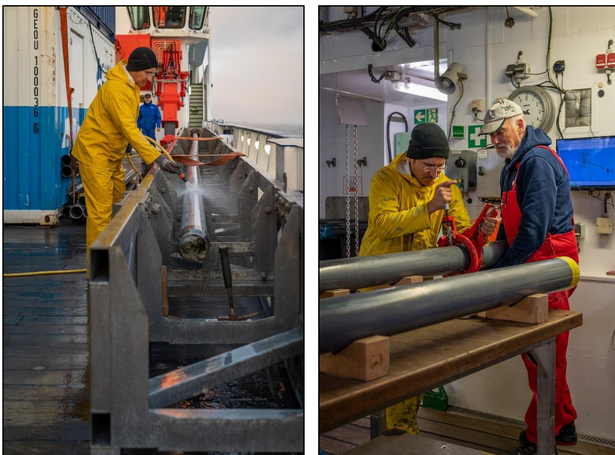
Fig. 5.5.5 Left: 18 m long gravity corer gets a wash after it arrived on deck. Right: After core liners were removed from the steel tube, they were cut into 1 m sections. Photo: Johan C. Faust
