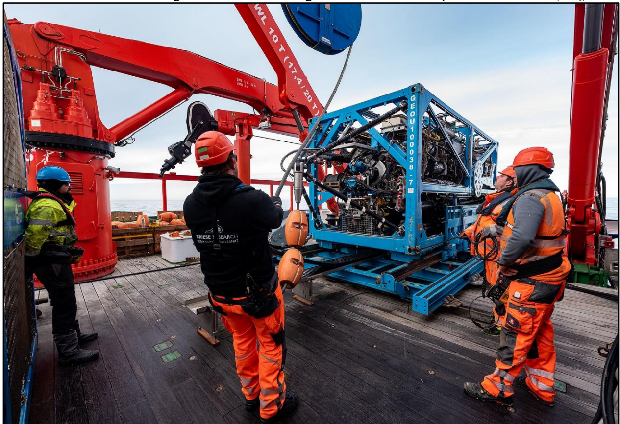
Fig. 5.5.6 Sea floor drill rig MARUM-MeBo200 on board R/V Maria S. Merian during expedition MSM 111. Photo: Volker Diekamp.
