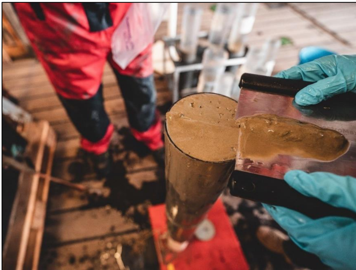
Fig. 5.5.3 Sampling a MUC using metal spatulas. Photo: Raphael Morard.
